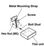
When your vehicle has the Bracket, mount the long hex bolt onto the rear panel of the CDA-9886R and put the Rubber Cap on the hex bolt. If your vehicle does not have the Mounting Support, reinforce the head unit with the metal mounting strap (not supplied). Connect all the leads of the CDA-9886R according to details described in the CONNECTIONS section.
